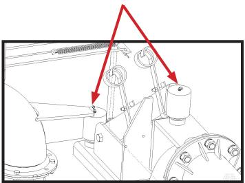
One post-season maintenance item on the swing arm is the elbow that gets the water from the parent machine to the swing span. The "U" pipe has a low pressure drain that can stick because the pressure never gets low enough to release the drain. Once the irrigation season is over, it is good practice to push the drain up and allow the water to drain so that it does not freeze and damage the system.
