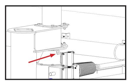
The last two grease zerks that are on the swing arm are located at the joint between the swing span and the hinge tower. They keep the ball greased so that the swing span can walk smoothly.
