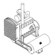
Note: The generator warranty requires that all combustion engines coupled to a generator, driving the system, must have a governor, a tachometer, and a safety load meter. The generator and system controls will be damaged by over or under engine speeding.
