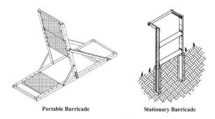
Note: These barricades are designed to be used on Reinke Systems, equipped with any auto-reverse or auto-stop option.
