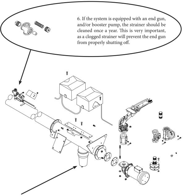
7. Check the sand trap regularly for accumulation of sand or debris. If the sand trap is full, clean it out with the trap off, start the pump to flush the system. (See instructions on page 44.) Replace the trap once it has flushed. The sand trap may need to be cleaned weekly if the water supply is dirty or the well is pumping a large amount of sand.
