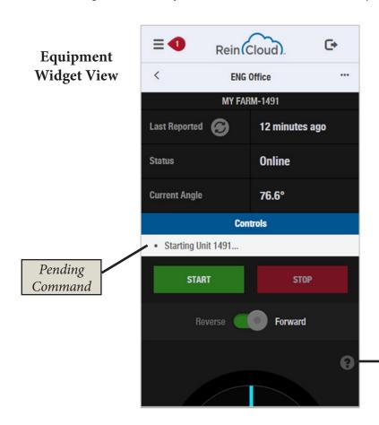
You will see the pending command under the Controls header until it is confirmed.
