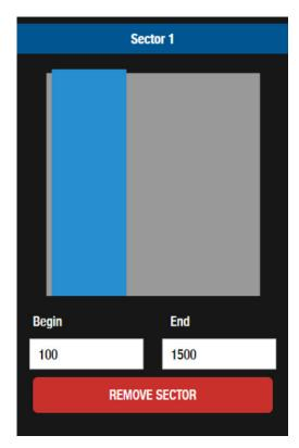
Select which control options you wish to perform with the sector by checking the box to enable the control. Choose the state of the control using the toggle or the input box provided. You can program the control in forward and in reverse.
