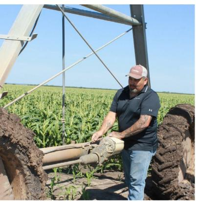
Inspect the drivetrain to ensure things are running smoothly during irrigation season.
