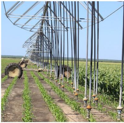
Check to make sure each tower is aligned.
