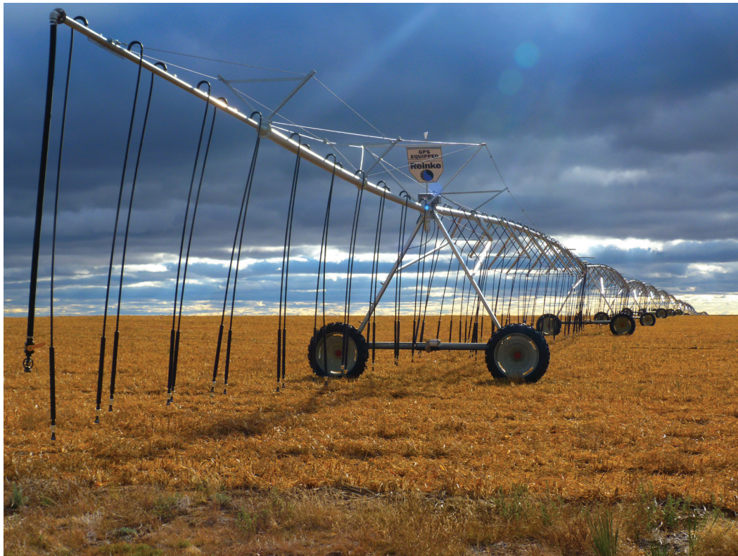
Park your pivot parallel with the winter winds and close all wheel tracks. Avoid parking next to the road to discourage cable theft.
