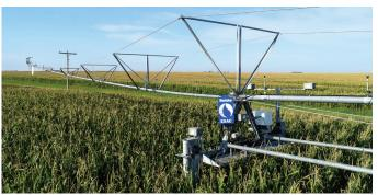
A Reinke swing arm corner with ESAC installed
