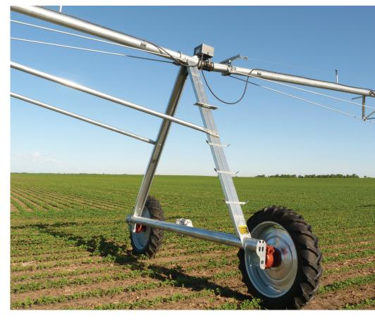
High-strength steel has been a proven foundation for our system's design. In the tower support design, high-strength steel used in the single C-channel leg eliminates the need for cross bracing between the tower legs, thus removing additional weight. That's why the single-leg tower always
