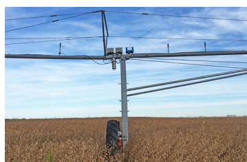
The RC10 hardware can connect to nearly any Reinke or competitive irrigation system.
