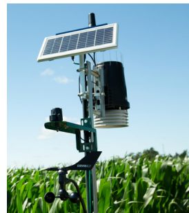
The RS300 collects data from compatible sensors that monitor soil moisture, weather variables and water meter readings and relays that data to the ReinCloud interface.
