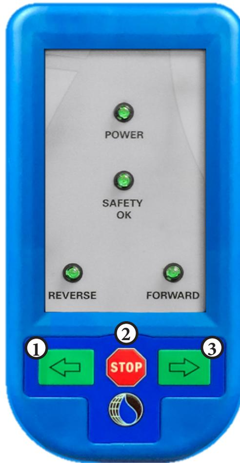
1. **Start Reverse:** Push to start the system in the reverse direction (counter-clockwise).
