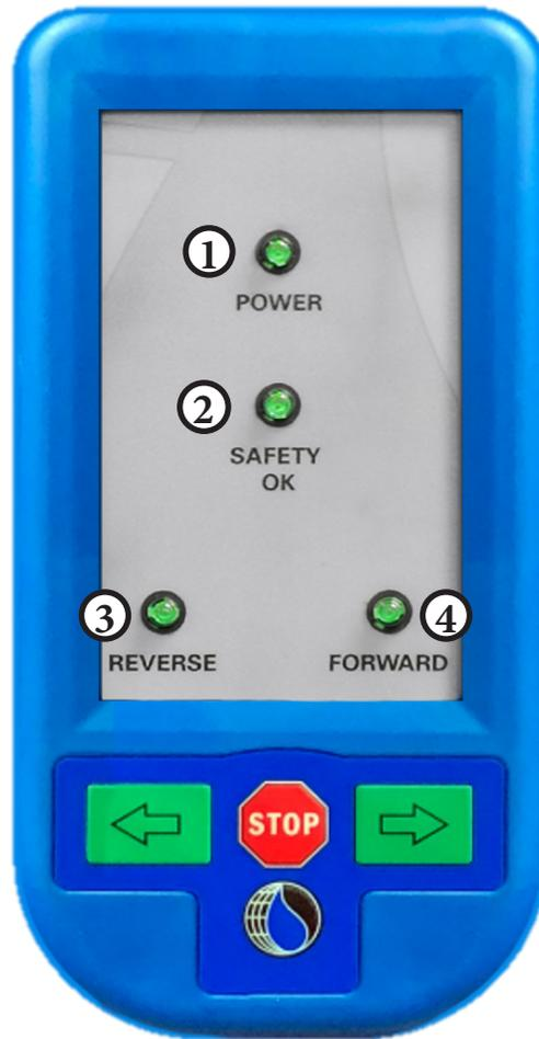
1. **System Power:** The LED will be illuminated when the main control panel is powered.
