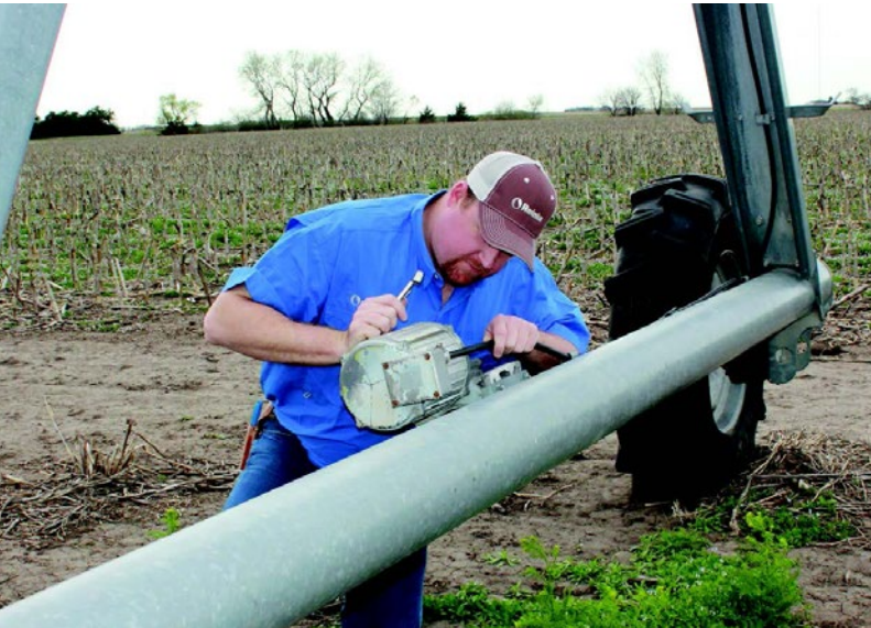
Inspect the drivetrain, including the center drive, wheel gears and tire pressure to make sure the pivot will move properly.
