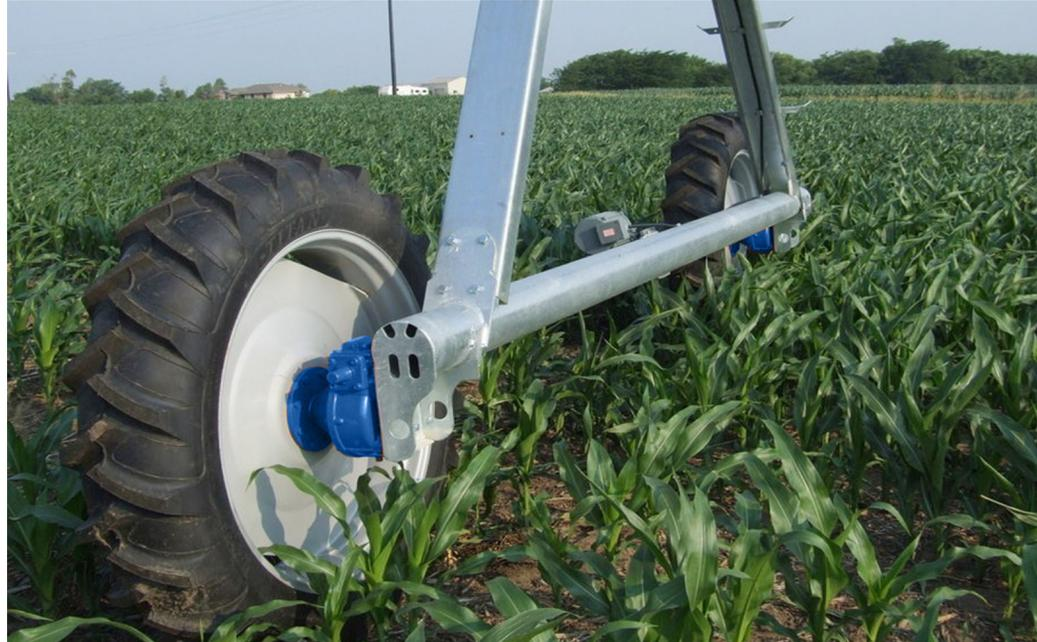
Reinke-UMC® 740-U-AD™ gearbox significantly outperformed its predecessor and experienced roughly half the amount of gear wear compared to its 8000 model competitor under the same test conditions.
