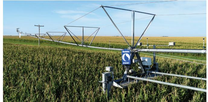
A Reinke swing arm corner with ESAC installed
